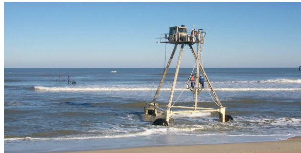
Figure 4. The Coastal Research Amphibious Buggy (CRAB) used for beach profile measurements at the U.S. Army Corps of Engineers Field Research Facility, Duck, North Carolina. Photo Credit
